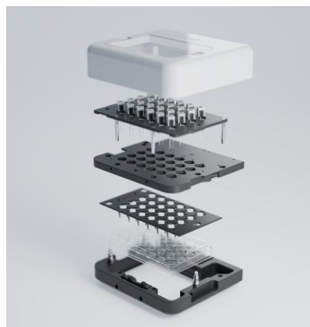
Figure 1: Cuore platform is designed to integrate long-term culturing of 3D engineered muscle tissue, with its electrical stimulation and contractility measurements enabling a broad range of assays.
