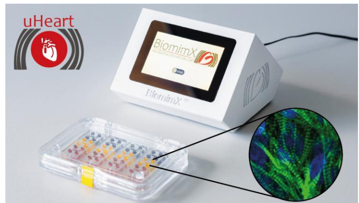
Figure 1. BiomimX experimental set-up used to generate atrial and ventricular beating heart-on-chip models (uHeart) exploiting iPSC-derived cardiomyocytes from Axol Bioscience.
